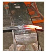
Step three: Round out the edges and draw out the beak.
