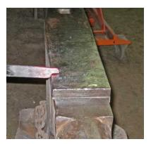
Step two: Using the far side of the anvil and half face blows you isolate the material for the head.
