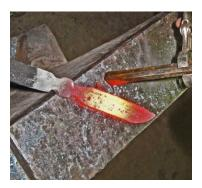
Step twelve: Make a second pass using your tool of choice to deepen the groove.
