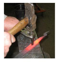
Step six: Drift the slot to round using increasing diameter drifts. The drifts are tapered at the ends so they can be driven through the hole.
