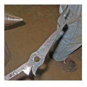
Step ten: Forge the end of the bar into a wing-like shape. For the next step you can use a chisel or make a lining tool. The lining tool allows you to line the long edge of the tool against the wing then strike it with a hammer so it creates a line that is always the same distance from the edge giving a smoother finish.
