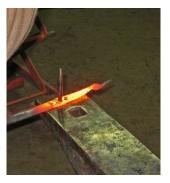
Step seven: Use half face strikes to start a tail, make sure the tail is going in the opposite direction of the beak.
